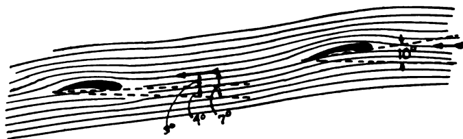
FIG. 1. DIAGRAM FROM EIFFEL TO SHOW DEVIATION OF STREAM-LINES BY "DOWN-WASH" OF WINGS.
